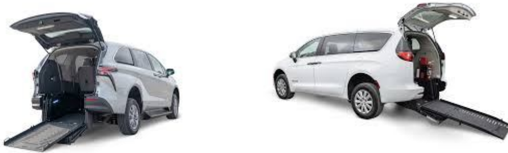
E. Ramp on Rear Side
