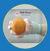
Robo Bionics is based at Maharashtra and their Product Grippy, Designed, engineered, and made in India is a 3D printed Prosthetic hand with a sense of touch and multi-grip control. It is alightweight battery-powered prosthesis for people with below elbow amputation age 15 years and above. They use chips that work at neuron level to detect correct signals for fingers.
