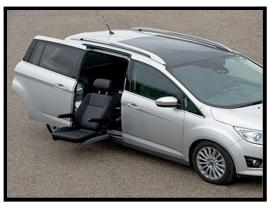
operated. <u>They are designed</u> to move the seat completely out of the vehicle to aid transfer and depending on specification can change the height of the seat to allow easy access.
