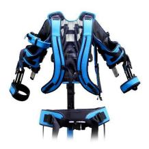
**EksoUE**, designed to assist the impacted arm and shoulder during clinical rehabilitation, helps patients with upper-extremity weakness or paralysis. It guides them in recovering strength, range of motion, and endurance.
